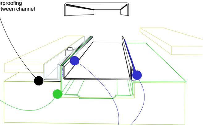
For all types of threshold installation ensure both sides of the channel are sealed before laying tile.
