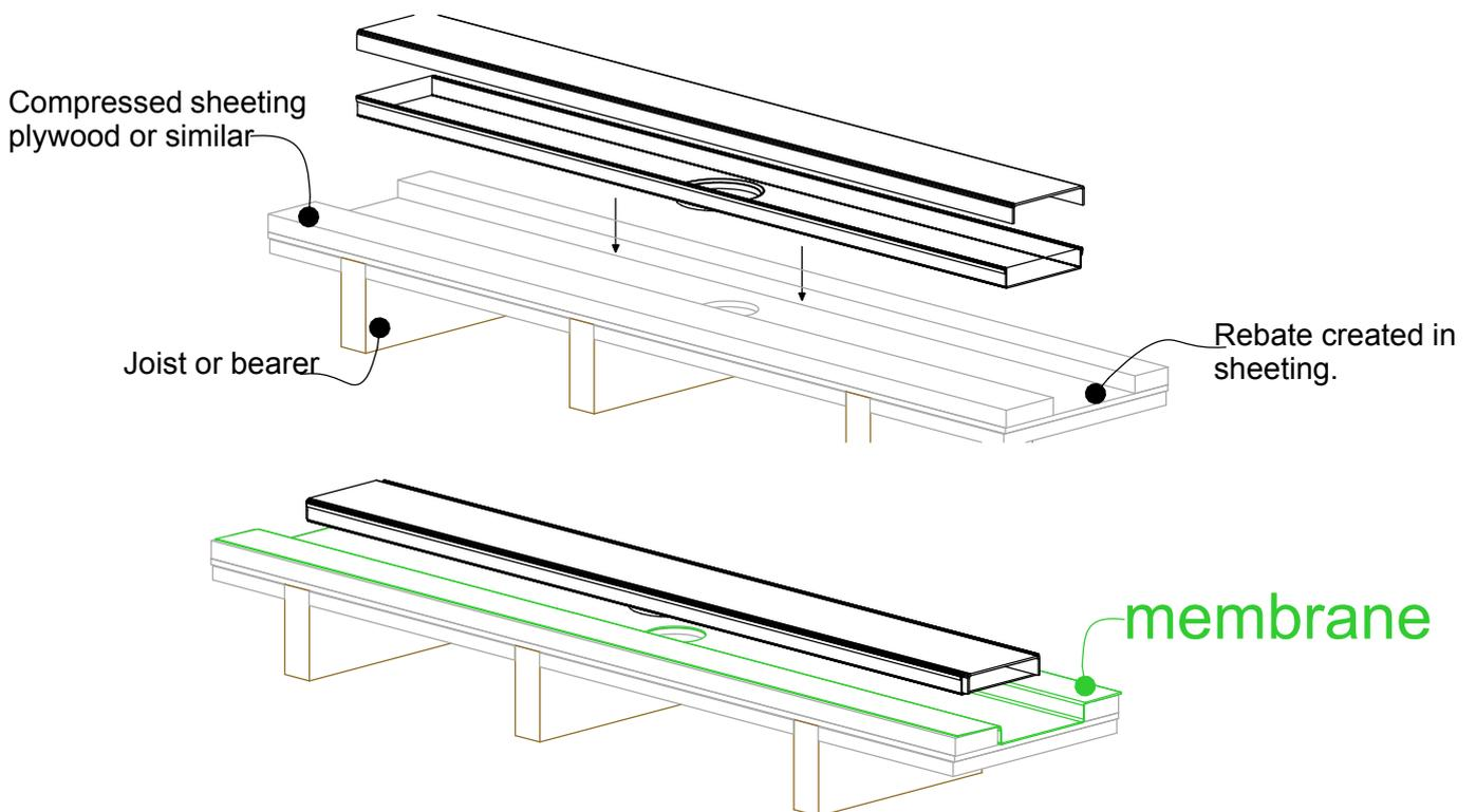
**NOTE: For exterior application allow for expansion of 1mm per metre by using quality suitable flexible sealant on channel joins.**
